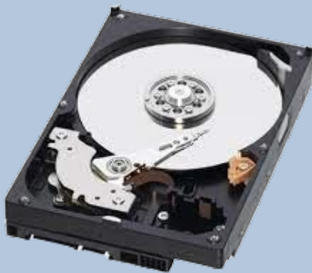
3.5" Hard drive with cover removed. Mechanical Hard Drive with spinning disk.
